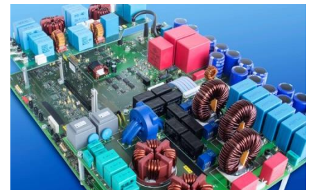
A 3-phase and 3-level multi-string PV inverter with dual-booster developed by the Power Electronics unit
